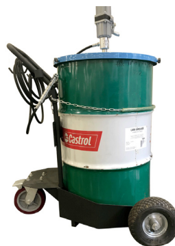
180 kg Mobile Grease Unit (pump, gun and hosing)
