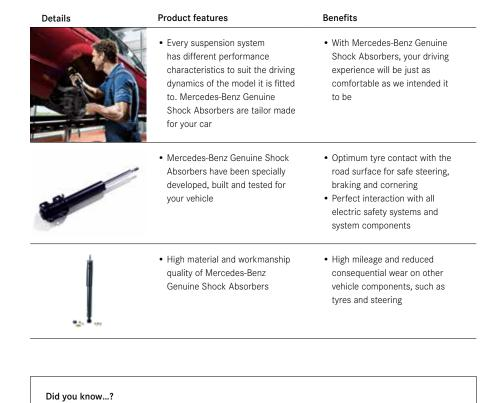
Worn shock absorbers increase braking distances.
