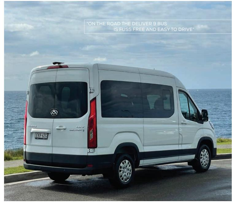
In terms of external dimensions the Deliver 9 11-seater bus measures 5546mm in length and has a 3366mm wheelbase. With the mid roof configuration as tested it has an overall height of 2545mm, while the payload limit for this particular test 11 seater bus was 1500 kilograms.
