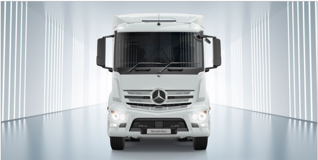
L-Cab ClassicSpace 2.30m with a 320mm engine tunnel
