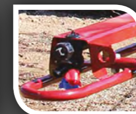
Fence line nozzles
