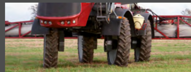
Crab steering – in difficult conditions and maneuvering
