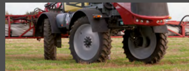
4-wheel steering – field mode
