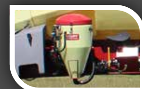
VACnMIX transfer hopper
