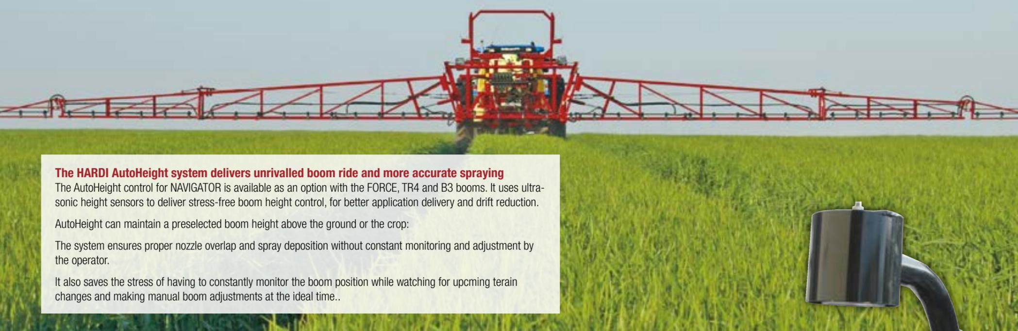
**The HARDI AutoHeight system delivers unrivalled boom ride and more accurate spraying**
