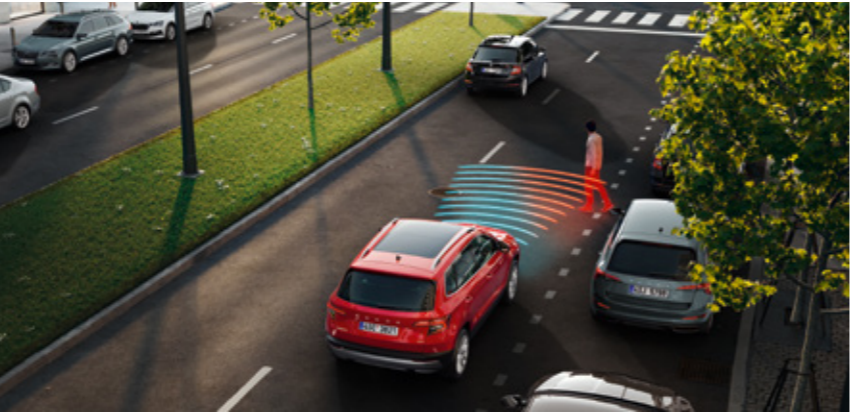
FRONT ASSIST WITH CITY EMERGENCY BRAKE o The Front Assist system, using a radar device in the front grille, is designed to monitor the distance from the vehicle ahead, including emergency braking function.
