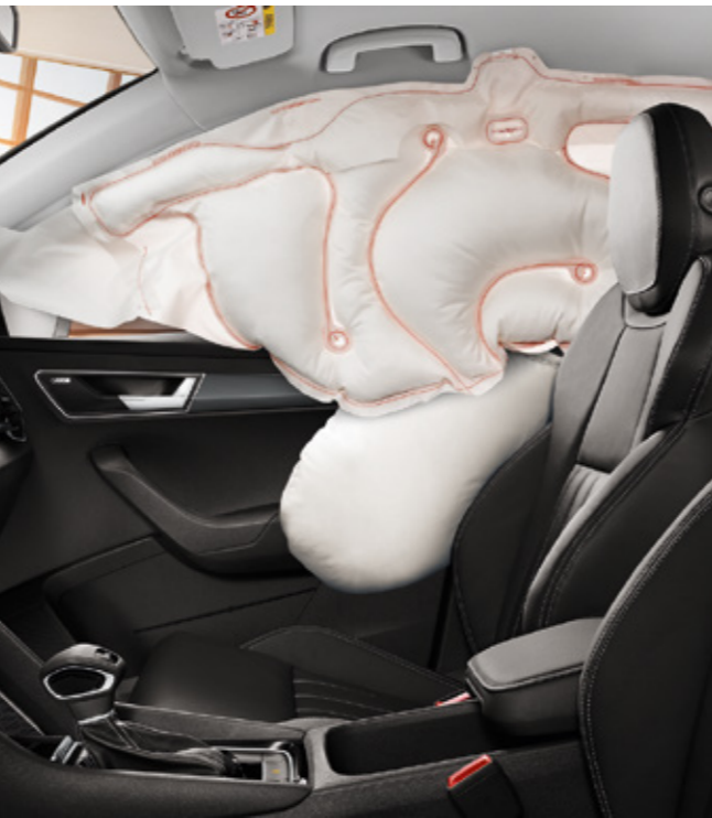
FRONT SIDE AIRBAGS Designed to protect front and rear occupants against serious head injury. The pelvis and chest of the driver and other passengers in the event of a side collision.
