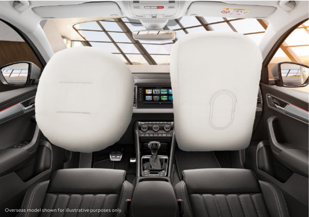
FRONT AIRBAGS The driver airbag is enclosed in the steering wheel and the passenger airbag is located in the dashboard.
