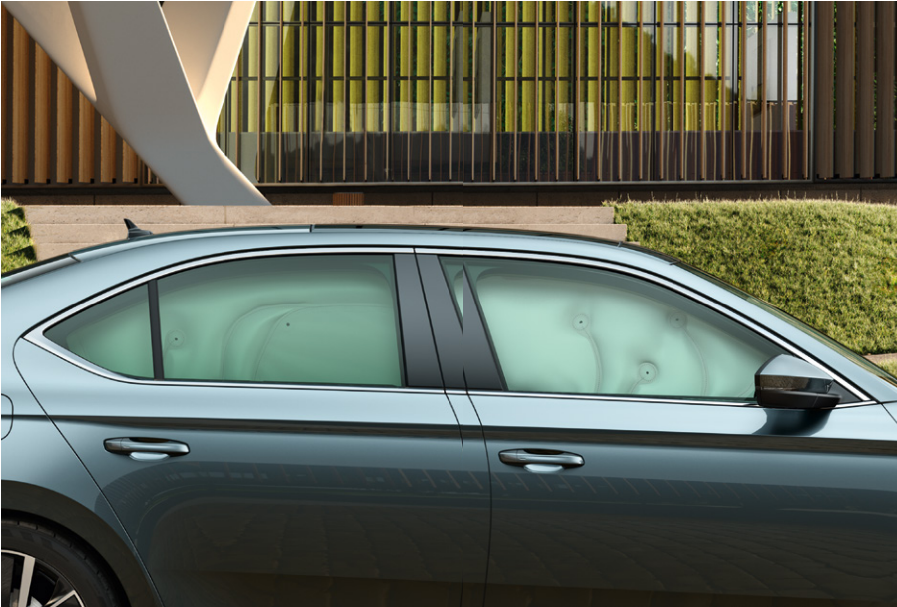
SIDE CURTAIN AIRBAGS Upon activation, side curtain airbags create a wall, which protects the front and rear occupants against head injury.
