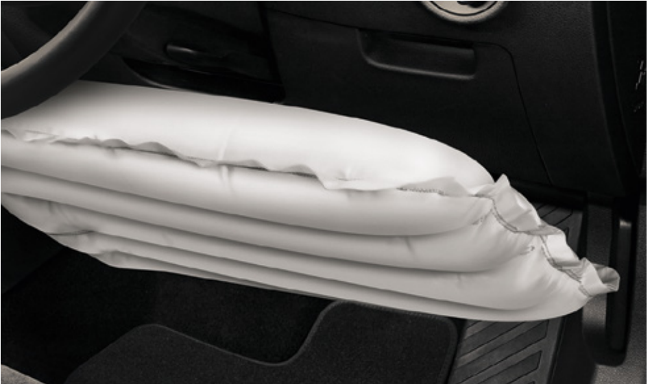
KNEE AIRBAG The knee airbag, which protects the driver's knees and shins, is located under the steering wheel.
