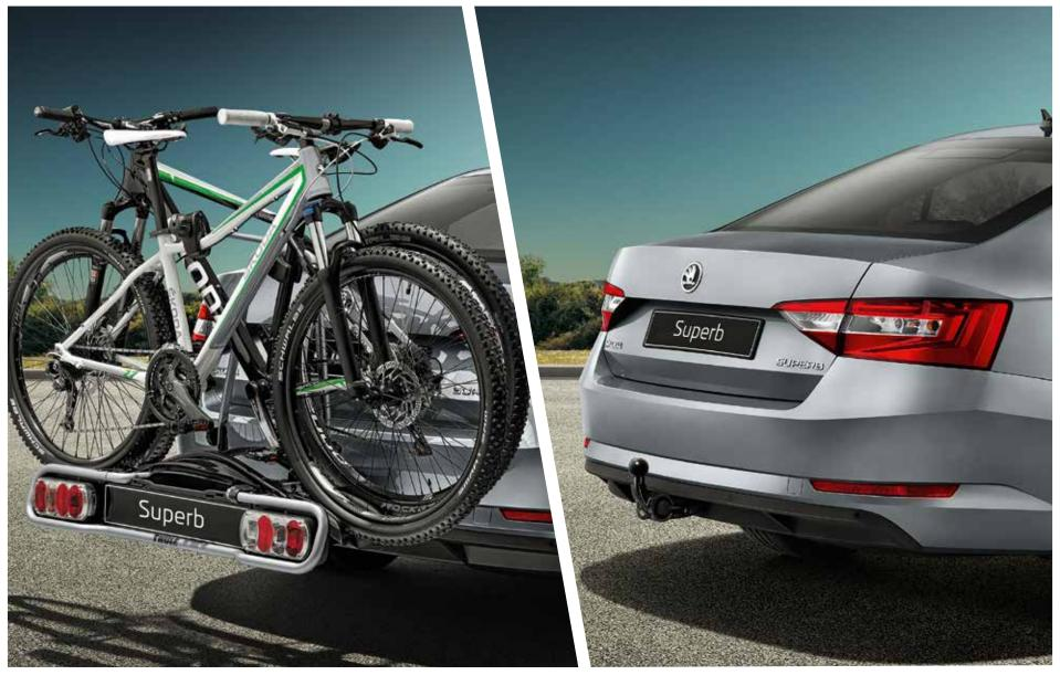
**Detachable tow bar with electrics** (overseas model shown) ŠKODA Genuine Accessories Detachable tow bar (3V0 092 155A) Electric wiring kit for cars with preparation (3V0 055 204A)
