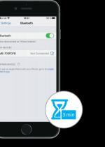
Add the device "MB-123456" or similar in your smartphone's Bluetooth® menu. The Bluetooth® link must be established within 3 minutes of inserting the Adapter. Otherwise, please re-insert the Adapter.
