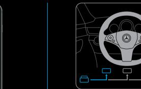
Insert the Mercedes me Adapter into the "OBD2 socket" in the driver's footwell once again.
