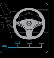
Insert the Mercedes me Adapter into your vehicle's diagnostics connector ("OBD2 socket"), which is located in the driver's footwell. In some vehicles. the cover of the OBD2 socket has to be opened beforehand for this purpose.
