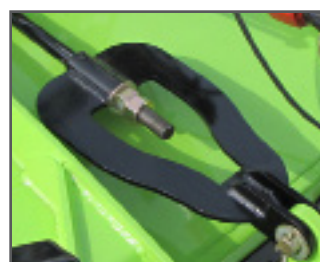
Single levelling rod with floating hitch
