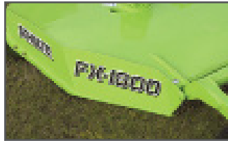
7 gauge Continuously Welded Single Domed Deck
