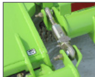
Greaseable adjustable turnbuckles for parallel levelling
