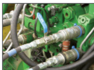
Ball valve wing lock up system
