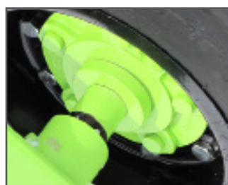
Metal seal guards on 517 hubs
