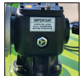
Convenient oil level site glass on gearboxes
