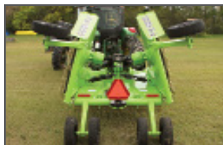
Narrow transport over-centering wing design
