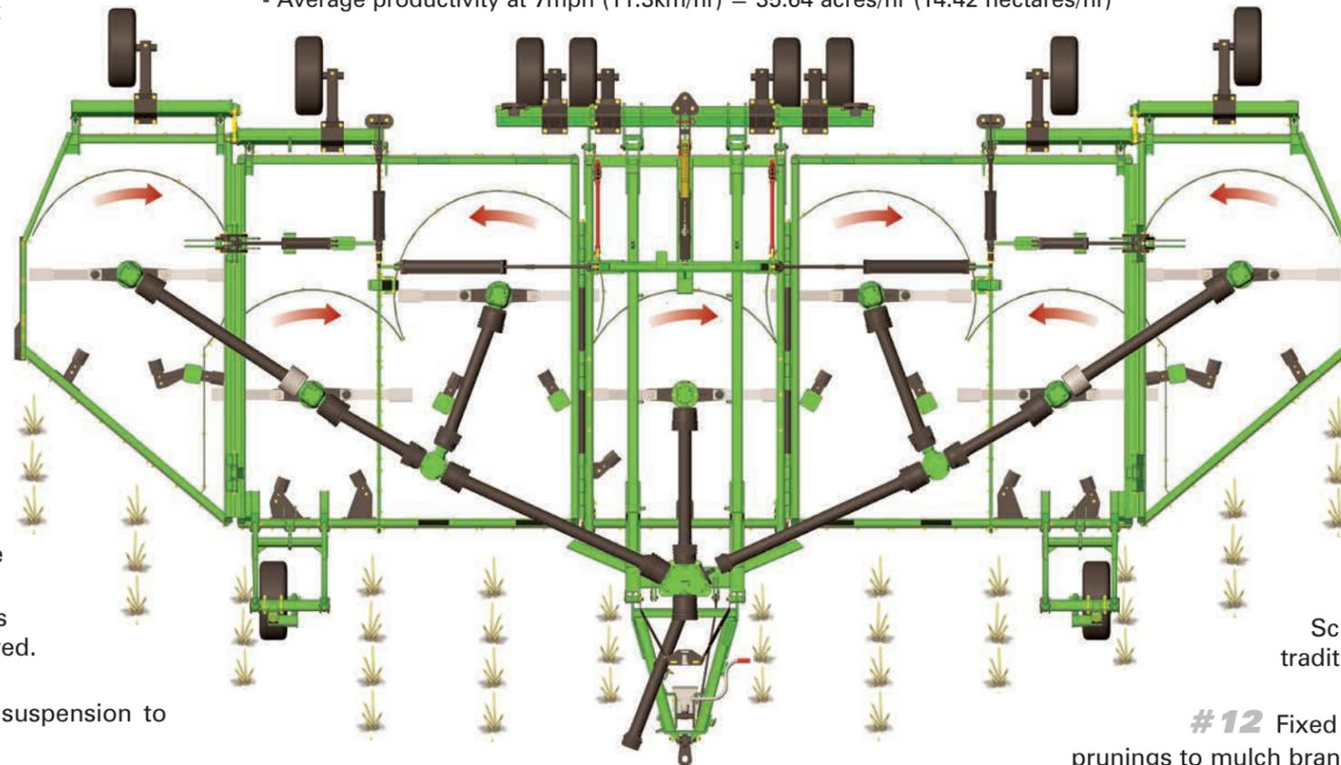
**#7** Schulte flex wing cutters are designed to work in most row crop spacings by using adjustable wheel standards or axle spindles.
