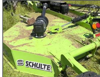
Continuously welded single domed deck
