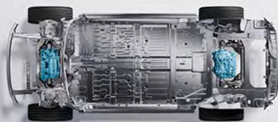
Front Double Wishbone + Independent Rear Five-link Suspension
