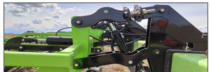
Hydraulic harrow control cylinder mounts between the parallel link arms and all pivot point use greaseless bushings for ease of service
