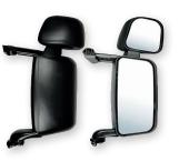
**OEM MIRROR** SUITS Scania • 4/R/P/T 2004 -Onwards • Electric & Heated • 650 x 290mm • Available in LH and RH
