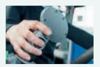
The button on the rear of the CommandGrip  $\ensuremath{^{\text{TM}}}$  give access to further functions.
