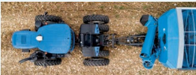
Grain cart applications with VF dual tyres (Row Crop Frame shown) allow for high-speed, low-pressure inflation, which lessens soil compaction while boosting fuel economy. Through less compaction, the T9 Series tractor improves your harvest and yields the following year.
