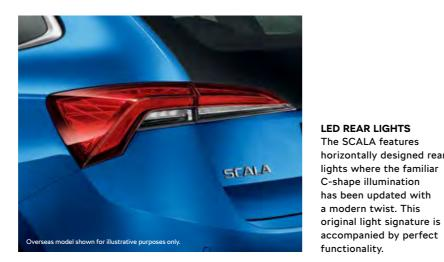
LED REAR LIGHTS The SCALA features horizontally designed rear lights where the familiar C-shape illumination has been updated with a modern twist. This
