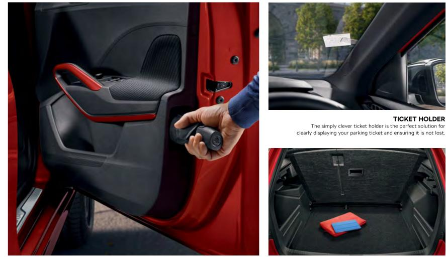
UMBRELLA IN DOOR An ingenious compartment integrated into the driver's door is designed to let water, retained from wet umbrella's, to drain away from the car. An original complimentary ŠKODA umbrella is also provided.
